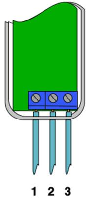
VCC + Ground terminals can be used to externally power the sensor with a 3.6V battery or special power adapter (which is not included in the scope of delivery). Digital + VCC is used to connect the external dry contact.
