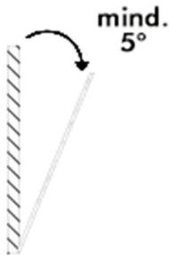
For German-style windows where the window sits on top of the window frame mounting on the side of the window is highly recommended. If no tilting detection is used, the sensor can be placed on any position of the door or the window. In case tilting detection is desired the sensor should be placed on the upper side of the window.
